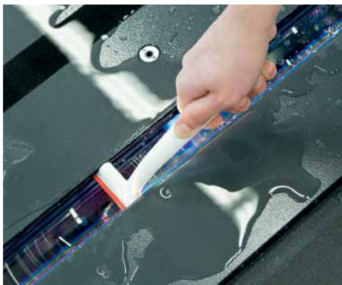
The measuring strip can be cleaned from the outside without opening mechanical components.
