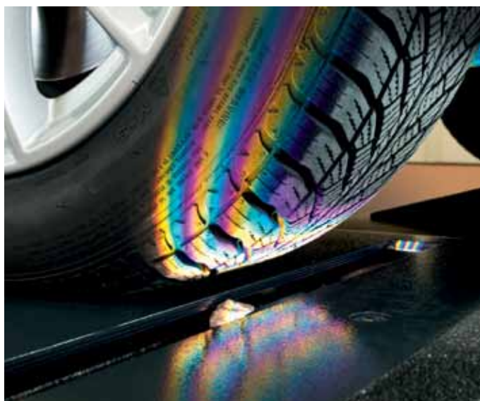
Small objects and soiling on the projection side have no effect on the measurement results.
