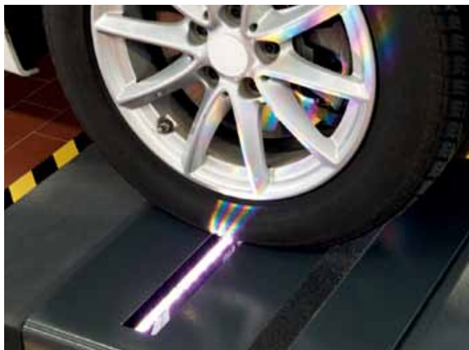
Measurements are based on color-coding – without any moving parts, without being affected by dust, vibration and moisture.
